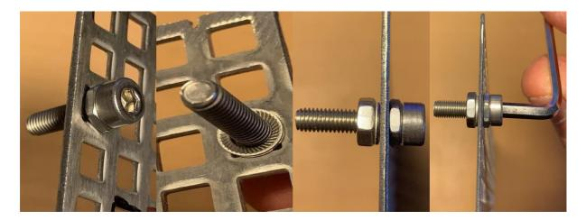
**Note**: It has been found that it is better to carry out all points from step 3 completely, column by column! A maximum of 4 screws are installed per column. So there is usually enough space to put on the open-end wrench when installing the screw.
