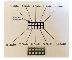
**2.4** Now insert your first coded screw through the hole in the top left. Then put a locking washer on the back of the thread and screw on a locking nut hand-tight.
