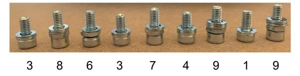
**2.3** Now take the position transmitter and the storage plate with the notch (top left) in hand and start screwing the 1st number in the top left of the first hole
