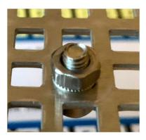
4.6 Take the 7mm jaws and the 3mm Allen wrench and tighten the screw (about 4-5Nm)
