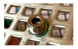
4.4 Take a lock washer out of the bag K and put it on the inserted therad
